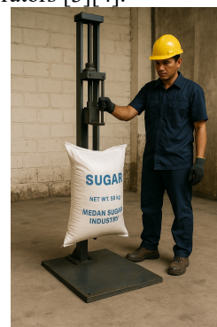
Figure 1 drop test process on 50 kg sugar packaging
