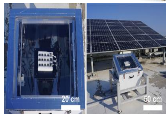
2 Figure: Outdoor Chamber Design for Radiative Cooling Measurement and SSC
