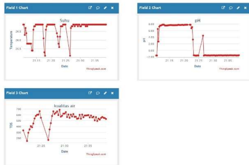
Figure 12 Temperature, pH, and TDS Curve on ThingSpeak
