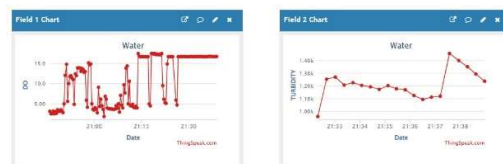
Figure 11 DO and Turbidity Curve on ThingSpeak
