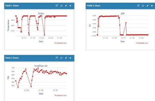
Figure 12 Temperature, pH, and TDS Curve on ThingSpeak
